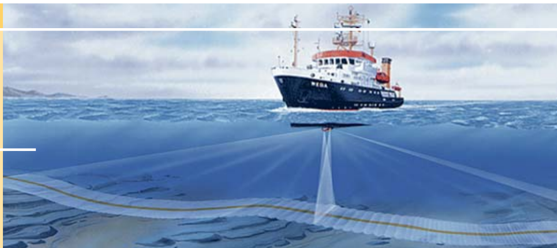
Fig. 10 Schematic depiction showing the recording of multibeam echo soundings made by the BSH's WEGA measurement, wreck search and research ship Source: BSH
