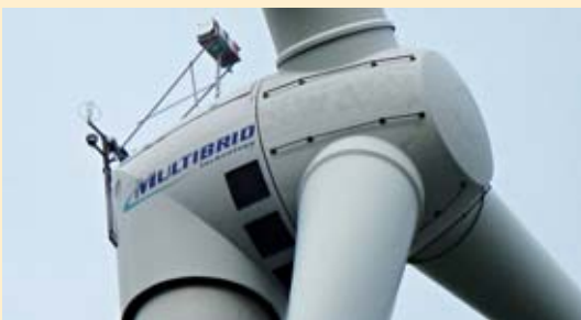
Fig. 12 Wind field measurements using LIDAR scanners Source: SWE, University of Stuttgart
