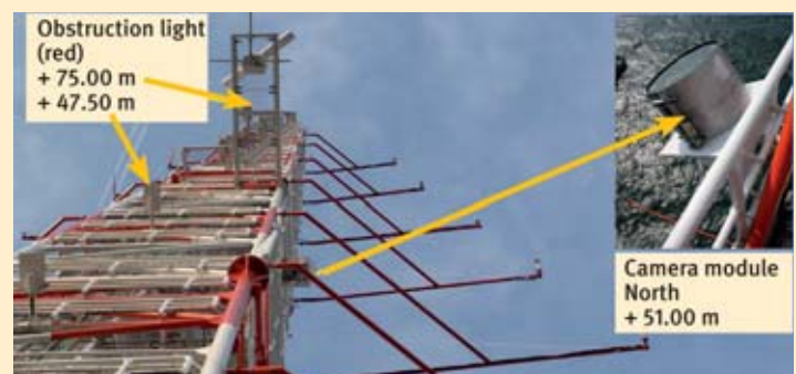
Fig. 20 Camera system for researching birds installed at a height of 51 metres on the north side of the measurement mast on FINO 2 Photo: GL – Garrad Hassan
