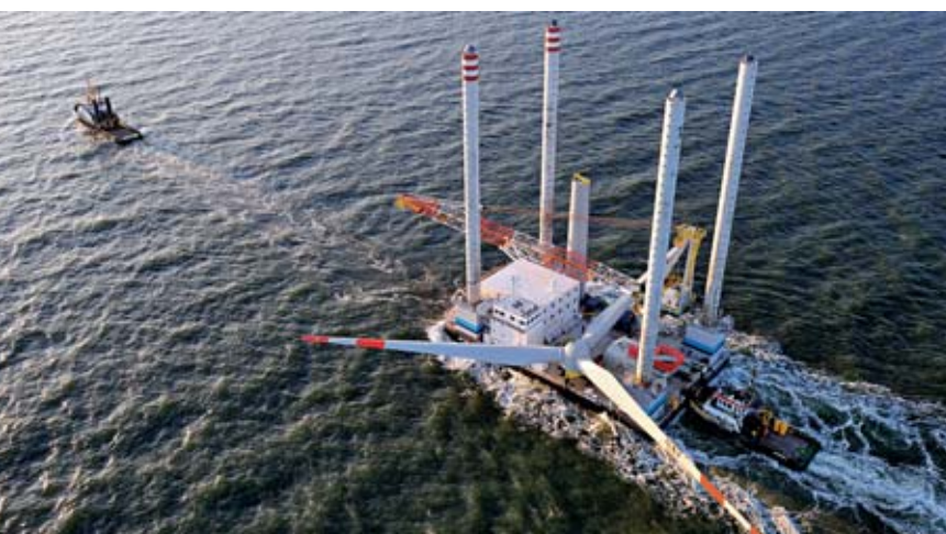
Fig. 8 Tugboats tow all the components to alpha ventus. Photo: DOTI 2009
