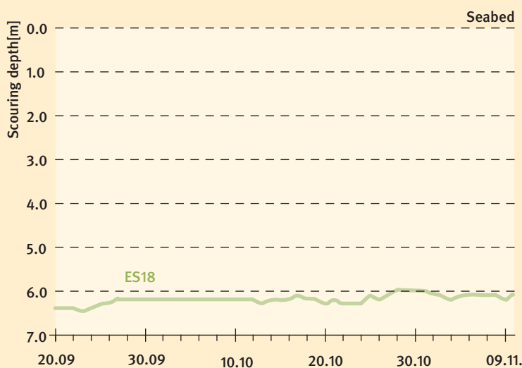
Fig. 23 Scouring depths recorded by the ES 18 echo sounder beneath the central segment in autumn 2010 Source: BSH
