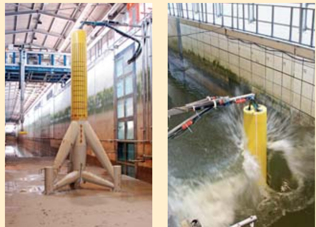
Fig. 31 A model of a tripod foundation is tested in the large wave channel. Photos: Franzius-Institut Hannover
