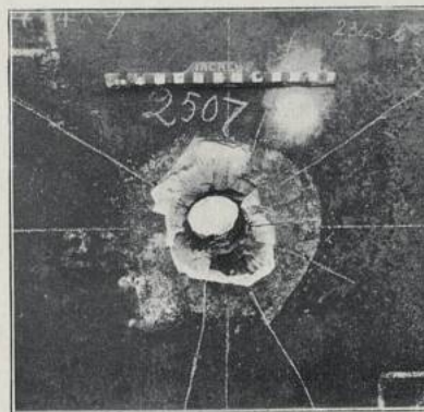
6-IN. ARMOUR-PIERCING SHOT versus 9-IN. COMPOUND PLATE. (Fired December 14th, 1888.)
