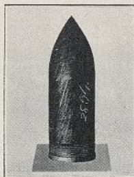
10-IN. ARMOUR-PIERCING SHOT versus 16-IN. COMPOUND PLATE.
