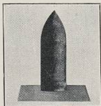
9.2-IN. ARMOUR-PIERCING SHOT versus 14-IN. COMPOUND PLATE.
