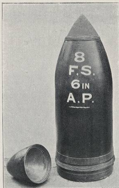
I. AND II. METHOD OF SECURING CAPPED SHOT III. SHOT AFTER PENETRATING KRUPP ARMOUR.
