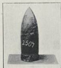
6-IN. ARMOUR-PIERCING SHOT versus 9-IN. COMPOUND PLATE. (Fired December 14th, 1888.)
