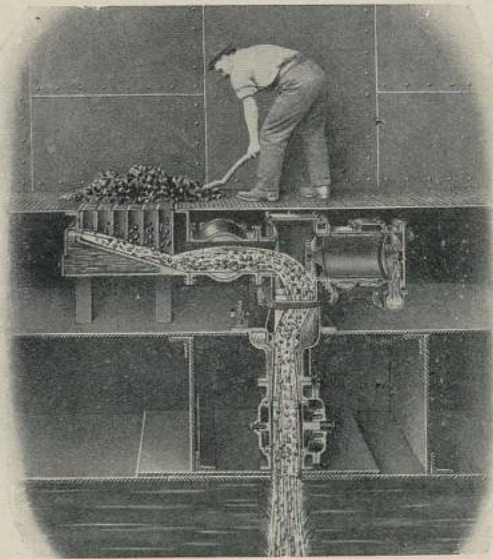
FIG. 55.—HYDRAULIC UNDERLINE ASH-EXPELLER.
