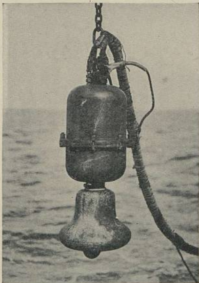
FIG. 75D.—LIGHT-VESSEL SUBMARINE BELL ON THE NORTH-WEST LIGHT-VESSEL.
