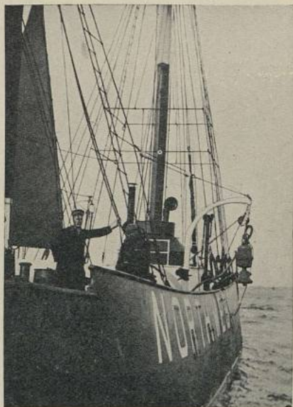
FIG. 75E.—NORTH-WEST LIGHT-VESSEL, SHOWING SUBMARINE BELL.
